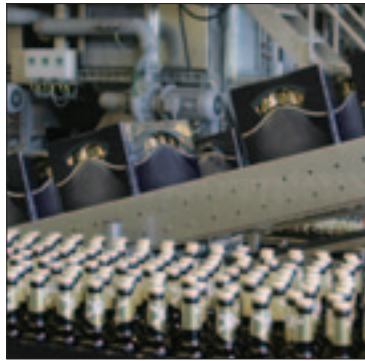
Production plant at a brewery equipped with sliding rails
